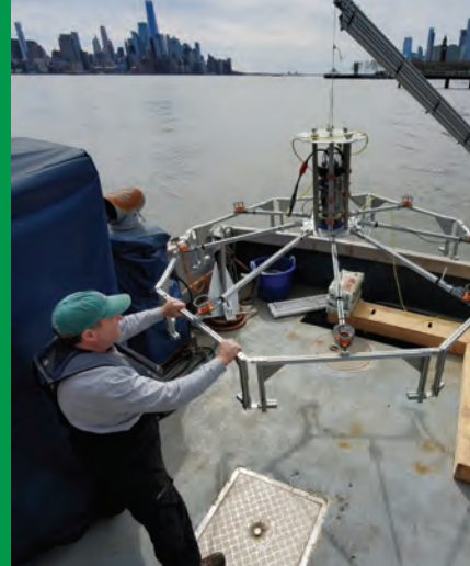
Stevens STAR Center researchers deploy a passive acoustic sensor in the Hudson River.
